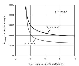
On-Resistance vs. Gate-to-Source Voltage
