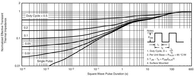
Normalized Thermal Transient Impedance, Junction-to-Ambient
