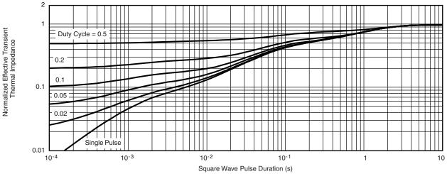
Normalized Thermal Transient Impedance, Junction-to-Foot
