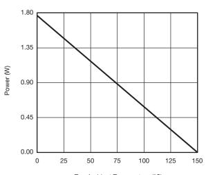
T<sub>A</sub> - Ambient Temperature (°C) **Power, Junction-to-Ambient**
