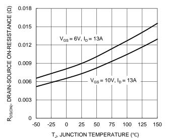
Figure 7. On-Resistance Variation with Junction Temperature
