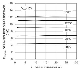
I<sub>D</sub>, DRAIN CURRENT (A) Figure 5. Typical On-Resistance vs. Drain Current and Temperature
