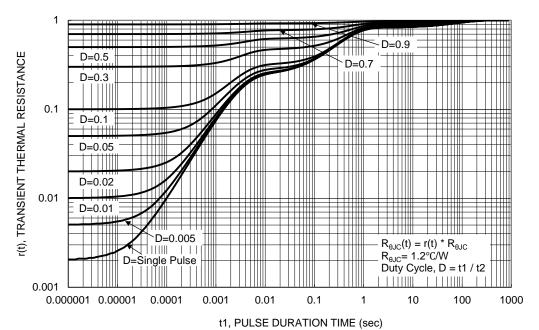
Figure 13. Transient Thermal Resistance
