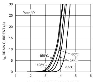
$V_{\rm GS}$ , GATE-SOURCE VOLTAGE (V) Figure 2. Typical Transfer Characteristic
