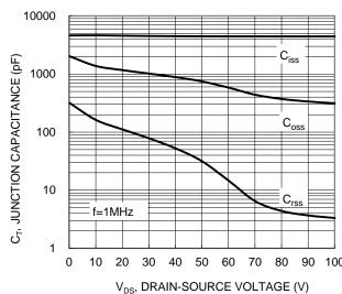
Figure 10. Typical Junction Capacitance
