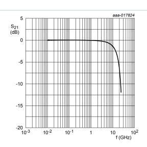
Fig. 6. Insertion loss; typical values
