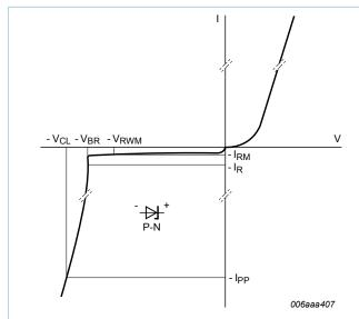
Fig. 3. V-I characteristics for unidirectional ESD protection diode
